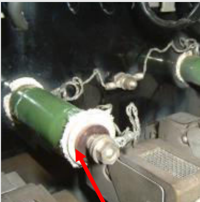
High Speed Circuit Breaker Resistors, Gasket
