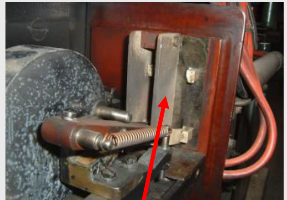
D.C. Circuit Breaker Auxiliary Relay (Clonker Box) – Cement Flash Guards
