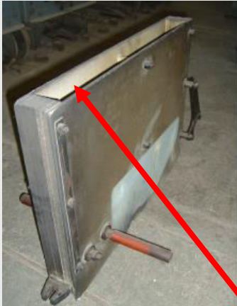
D.C. Circuit Breaker Arc Chute
